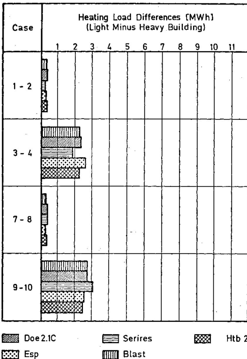
**fig. 21** Differences in annual heating loads of Phase I between light and heavyweight buildings calculated by detailed building energy analysis simulation models with weather conditions of DENVER.
