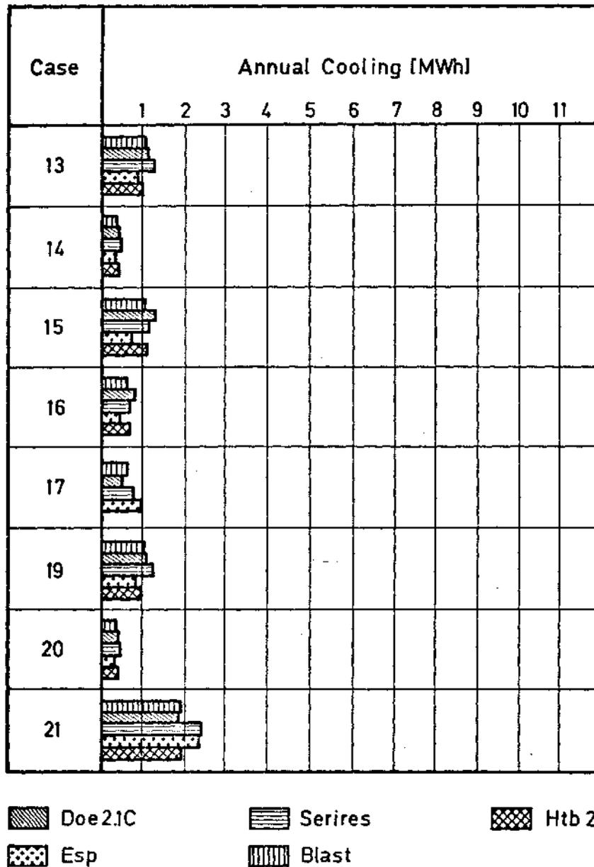
**Fig. 26** Annual cooling loads of Phase II calculated by detailed building energy analysis simulation models with weather conditions of DENVER.
