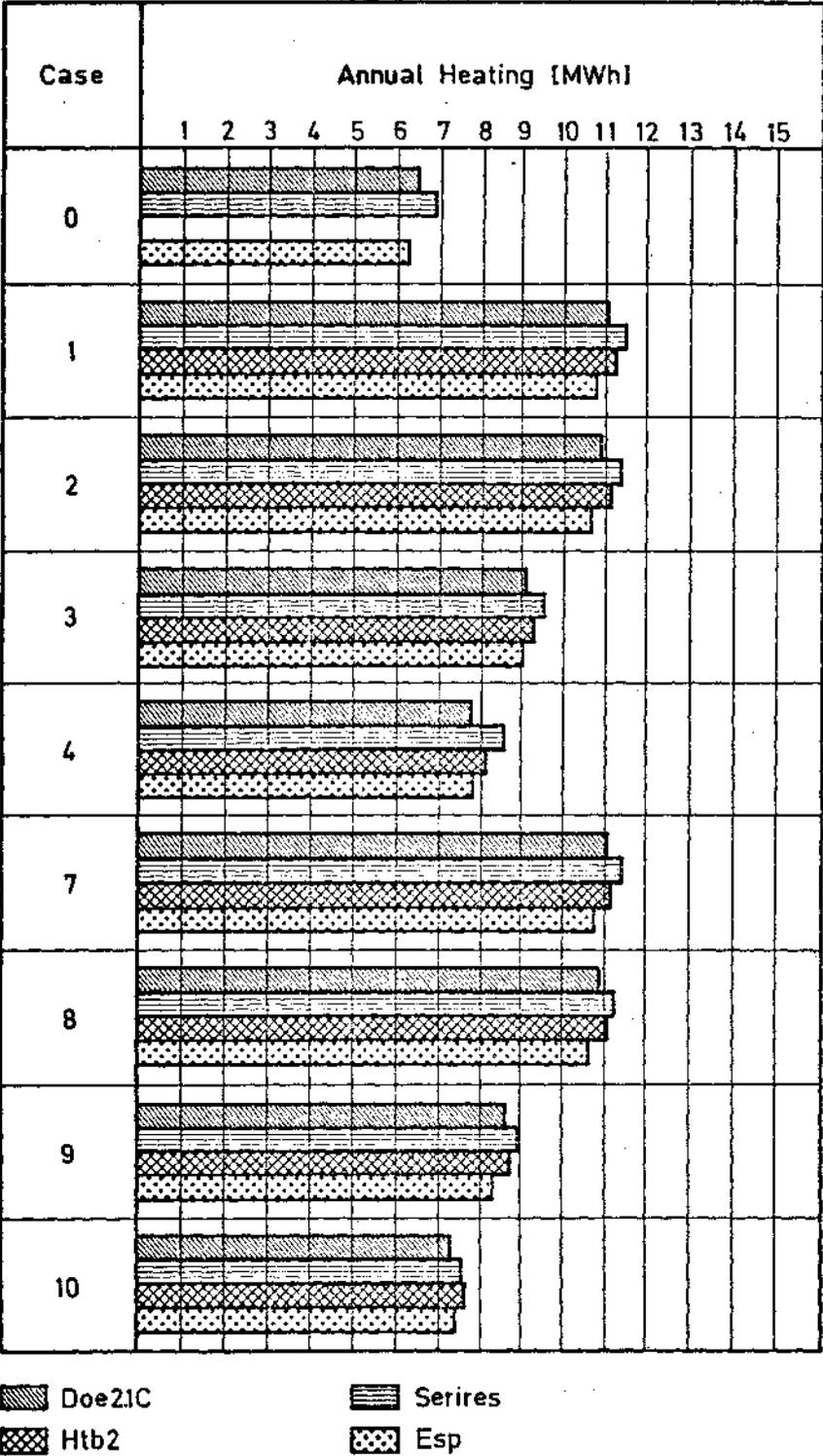
**Fig. 3** Annual heating loads of Phase I calculated by detailed building energy analysis simulation models with weather conditions of COPENHAGEN.
