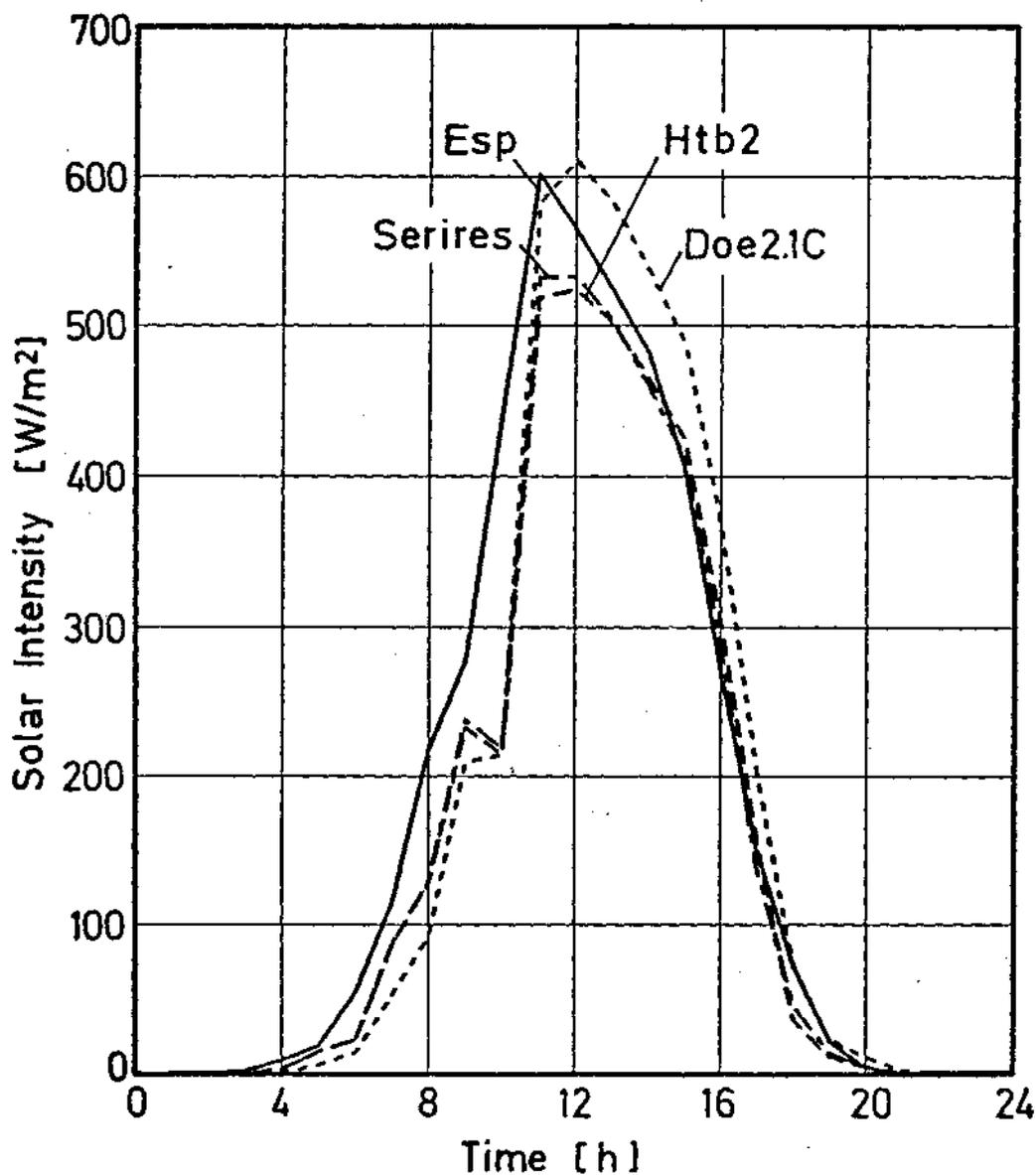
**Fig. 10** Hourly solar radiation incident on the external south facing surface calculated by detailed building energy analysis simulation models with weather conditions of COPENHAGEN, May 30.
