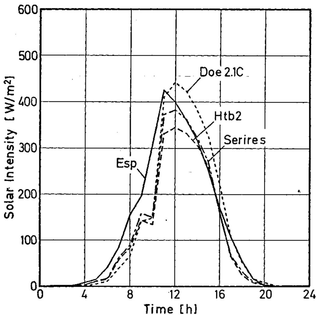
**Fig. 12** Hourly solar gain into building of Cases 3-4 and 9-12 calculated by detailed building energy analysis simulation models with weather conditions of COPENHAGEN, May 30.
