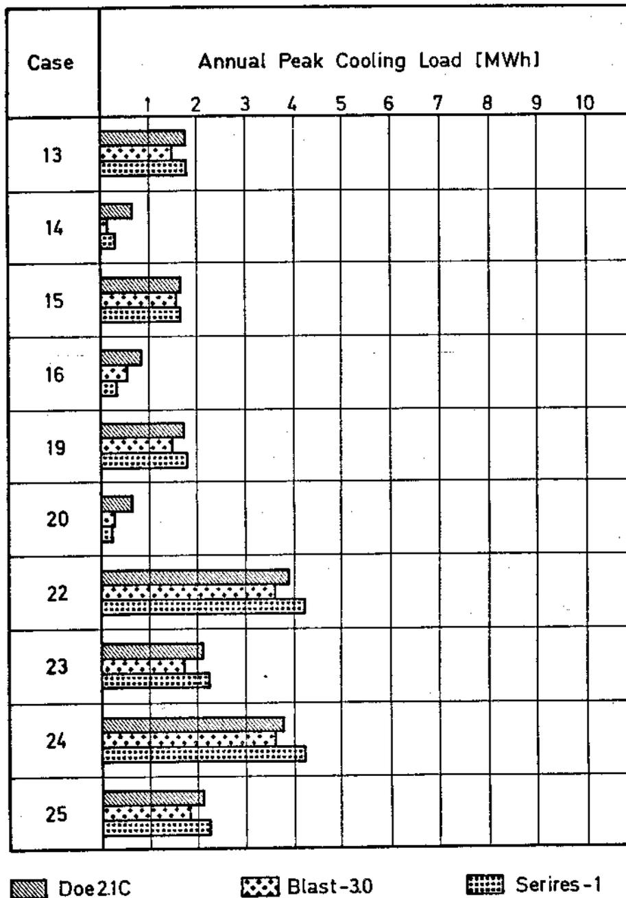
**Fig. 41** Annual peak cooling loads of Phase II calculated by detailed building energy analysis simulation models with weather conditions of COPENHAGEN.
