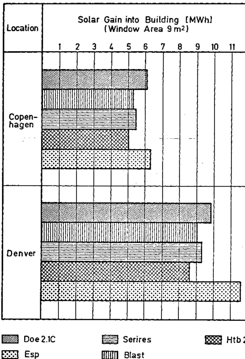
**Fig. 8** Annual solar input of cases with window area 9 m' calculated by detailed building energy analysis simulation models with weather conditions of COPENHAGEN and DENVER.
