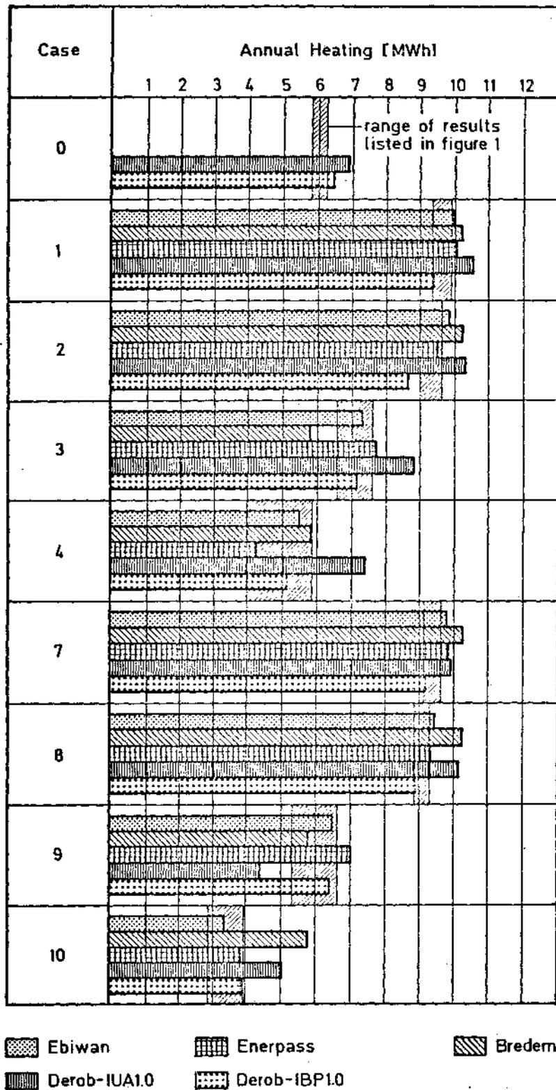
**Fig. 17** Annual heating loads of Phase I calculated by design tools with weather conditions of DENVER. Hatched areas indicate the ranges of results obtained by detailed building energy analysis simulation models (BLAST, DOE 2.1C, SERIRES, HTB 2, ESP) in Fig. 1.
