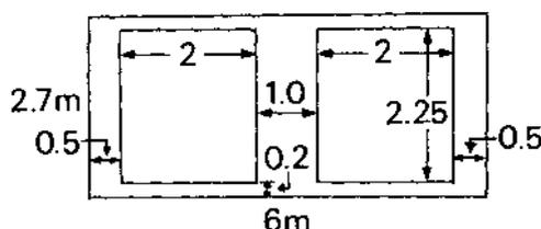
Figure A2: Glazing on South wall.
