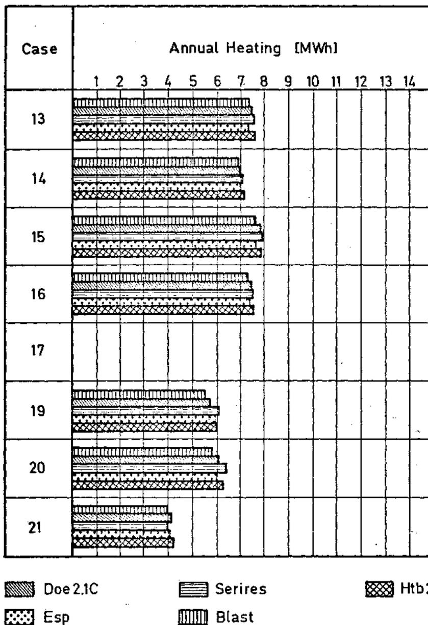
**Fig. 27** Annual heating loads of Phase II calculated by detailed building energy analysis simulation models with weather conditions of COPENHAGEN.
