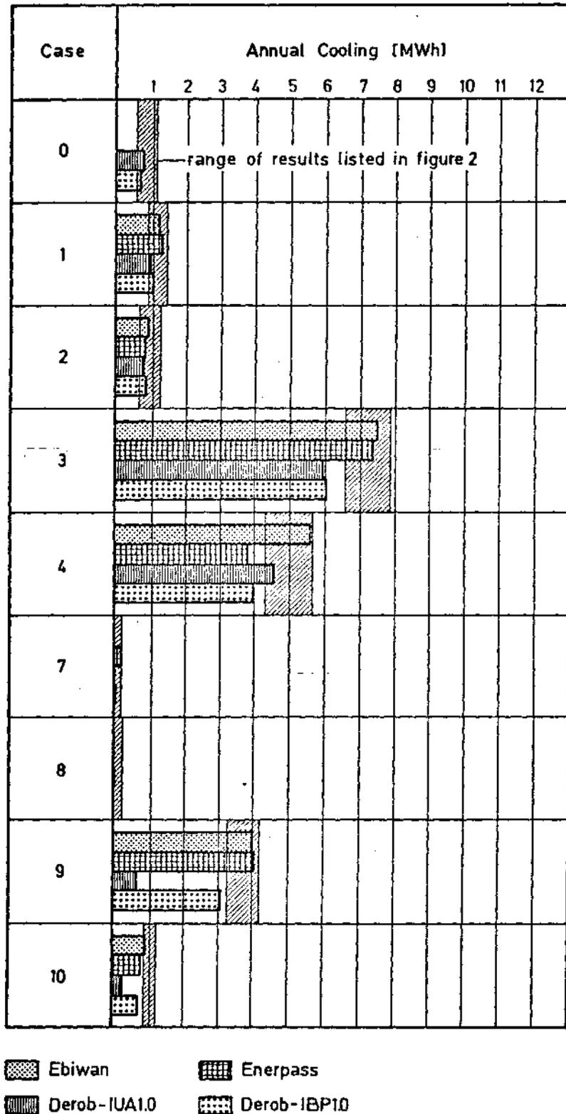
**Fig. 18** Annual cooling loads of Phase I calculated by design tools with weather conditions of DENVER. Hatched areas indicate the ranges of results obtained by detailed building energy analysis simulation models (BLAST, DOE 2:1C, SERIRES, HTB 2, ESP) in Fig. 2.
