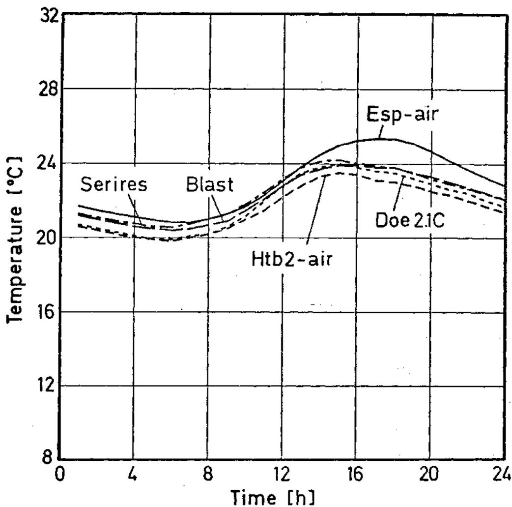
**Fig. 15** Hourly free-floating temperatures of Case 12 (heavyweight building) calculated by detailed building energy analysis simulation models with weather conditions of DENVER, May 30.
