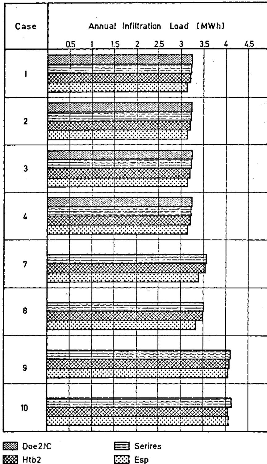
**Fig. 6** Annual infiltration loads of Phase I calculated by detailed building energy analysis simulation models with weather conditions of DENVER.
