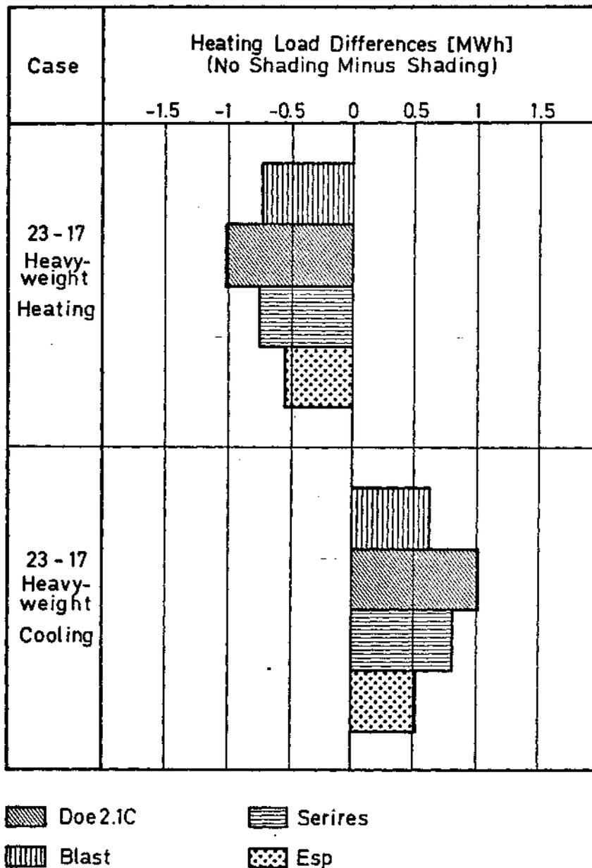
**Fig. 34** Differences in annual heating loads of Phase II between no shading and shading calculated by detailed building energy analysis simulation models with weather conditions of DENVER.
