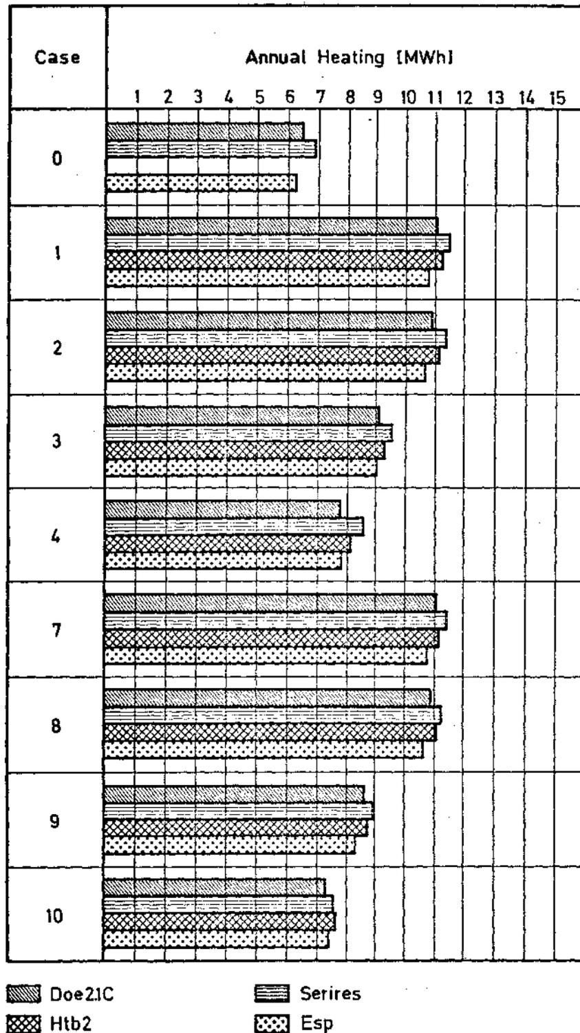
**Fig. 3** Annual heating loads of Phase I calculated by detailed building energy analysis simulation models with weather conditions of COPENHAGEN.
