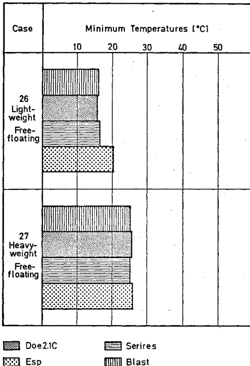
**Fig. 37** Minimum daily free-floating temperatures of Case 26 (light-weight) and Case 27 (heavyweight building) calculated by detailed building energy analysis simulation models with weather conditions of DENVER, October 17.
