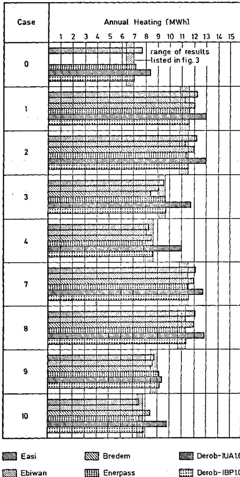
**fig. 19** Annual heating loads of Phase I calculated by design tools with weather conditions of COPENHAGEN. Hatched areas indicate the ranges of results obtained by detailed building energy analysis simulation models (BLAST, DOE 2.1C, SERIRES, HTB 2 , ESP) in Fig. 3.
