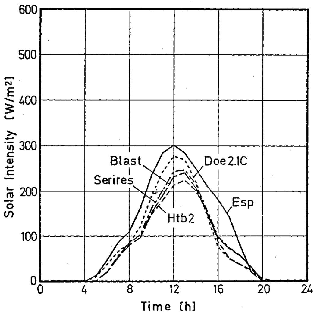
**fig. 11** Hourly solar gain into building of Cases 3-4 and 9-12 calculated by detailed building energy analysis simulation models with weather conditions of DENVER, May 30.
