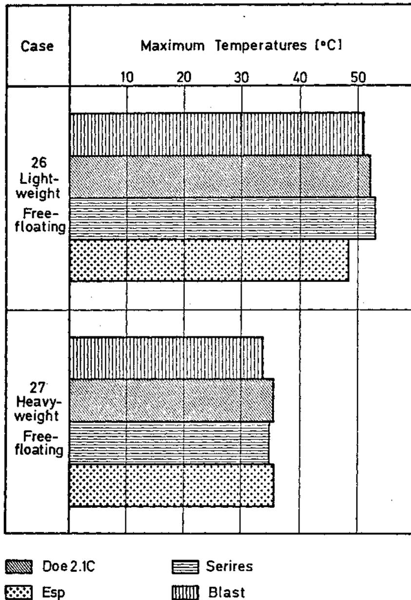
**Fig. 36** Maximum daily free-floating temperatures of Case 26 (light-weight) and Case 27 (heavyweight building) calculated by detailed building energy analysis simulation models with weather conditions of DENVER, October 17.
