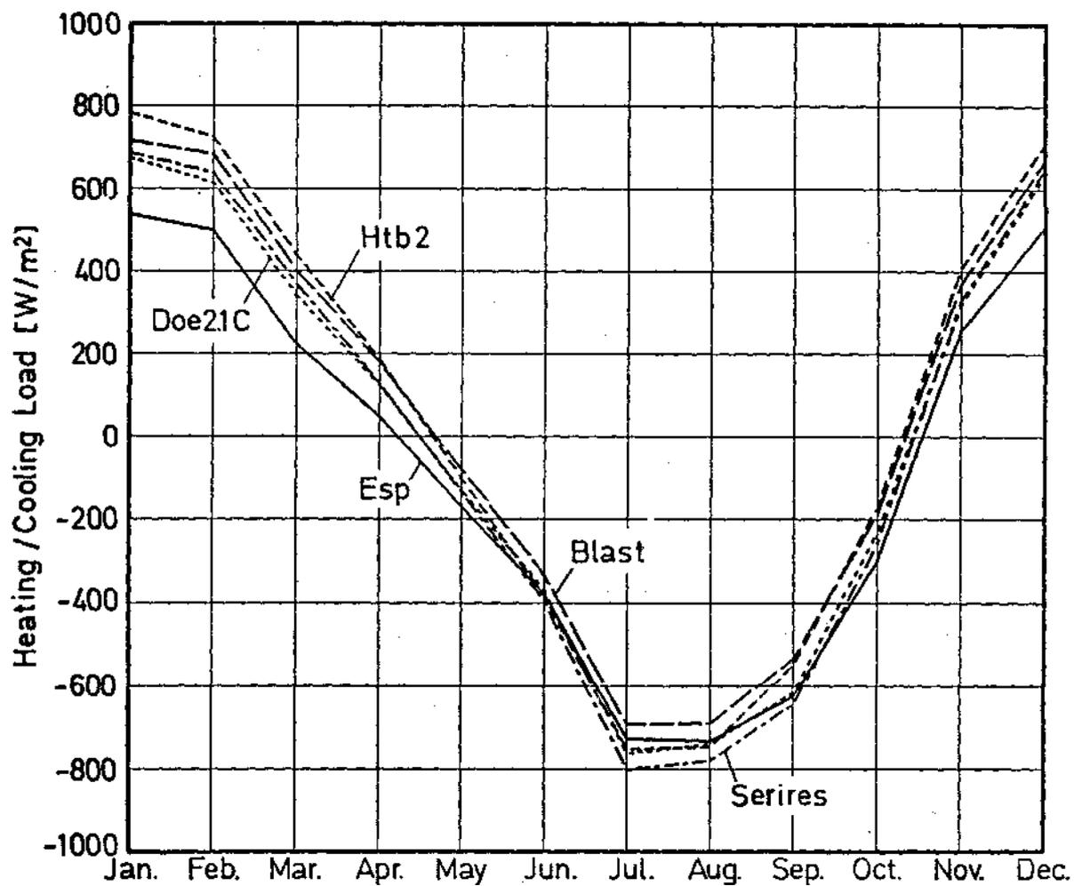
**Fig. 5** Monthly net plant loads of Case 4 calculated by detailed building energy analysis simulation models with weather conditions of DENVER.
