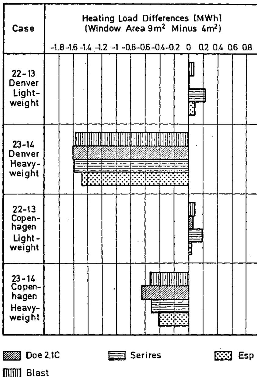
**Fig. 35** Differences in annual heating loads of Phase II between 9 m' and 4 m' south window area calculated by detailed building energy analysis simulation models with weather conditions of DENVER and COPENHAGEN.
