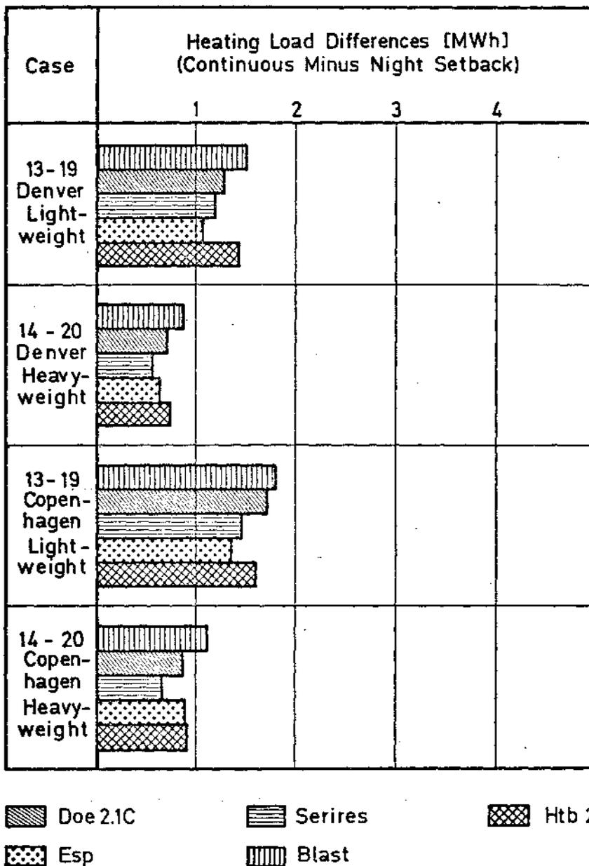
**Fig. 33** Differences in annual heating loads of Phase II between continuous and night setback heating modes calculated by detailed building energy analysis simulation models with weather conditions of DENVER and COPENHAGEN.
