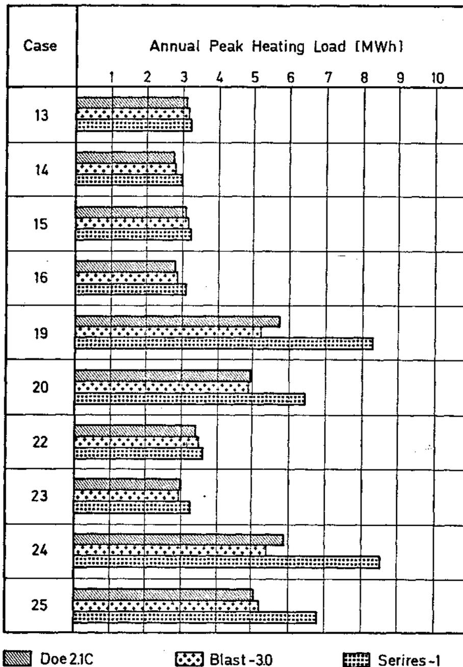
Fig. 40 Annual peak heating loads of Phase II calculated by detailed building energy analysis simulation models with weather conditions of COPENHAGEN.
