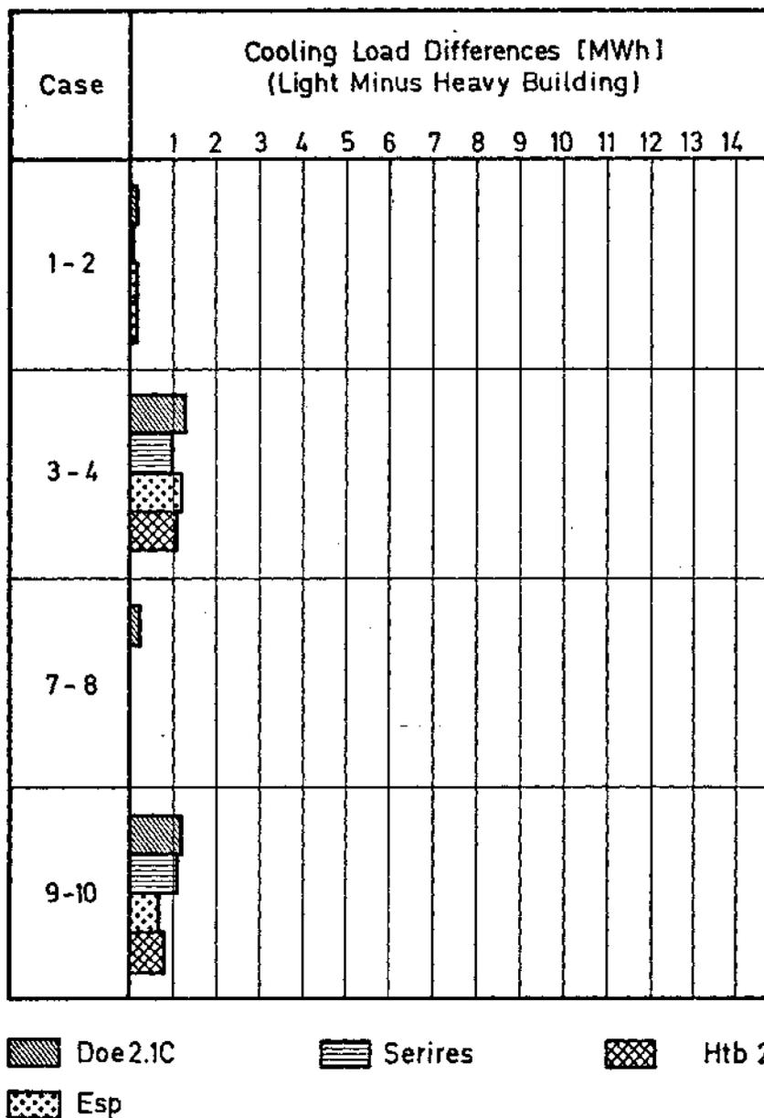
**Fig. 24** Differences in annual cooling loads of Phase I between light and heavyweight buildings calculated by detailed building energy analysis simulation models with weather conditions of COPENHAGEN.
