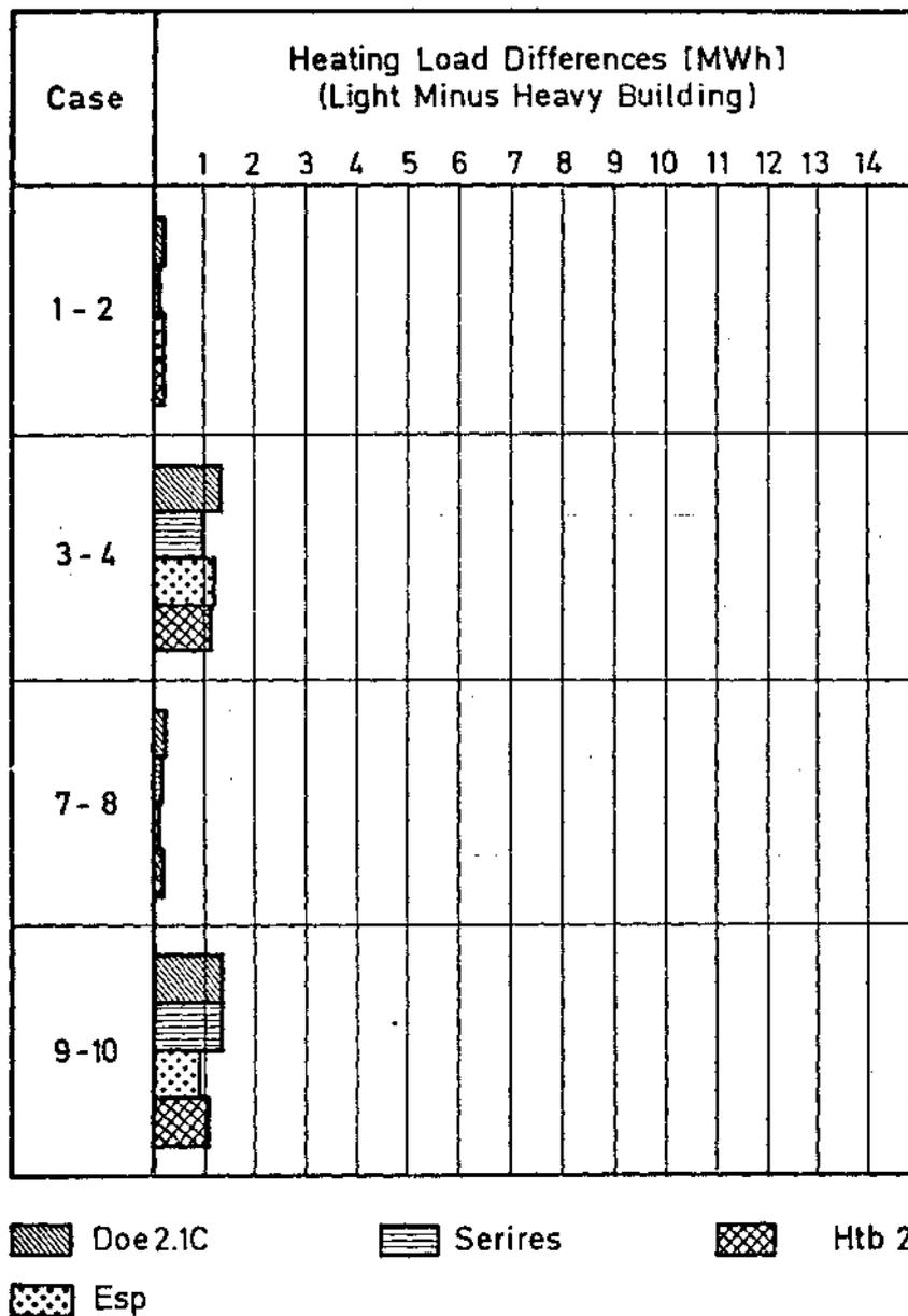
Fig. 23 Differences in annual heating loads-of Phase I between light and heavyweight buildings calculated by detailed building energy analysis simulation models with weather conditions of COPENHAGEN.
