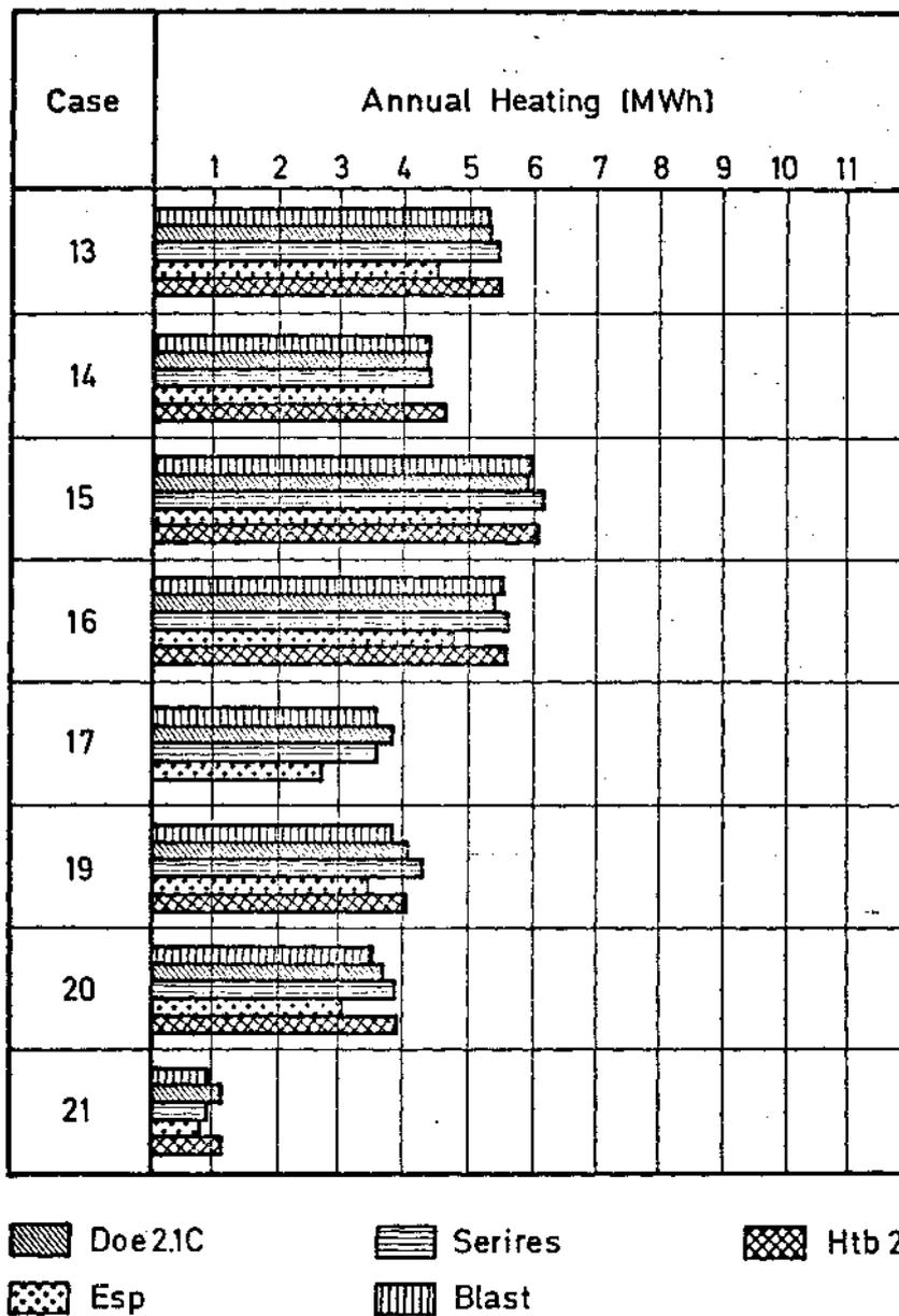
**Fig. 25** Annual heating loads of Phase II calculated by detailed building energy analysis simulation models with weather conditions of DENVER.
