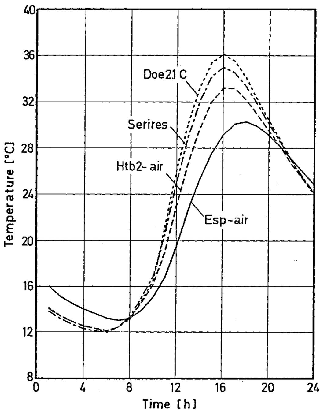
**Fig. 14** Hourly free-floating temperatures of Case 11 (lightweight building) calculated by detailed building energy analysis simulation models with weather conditions of COPENHAGEN, May 30.
