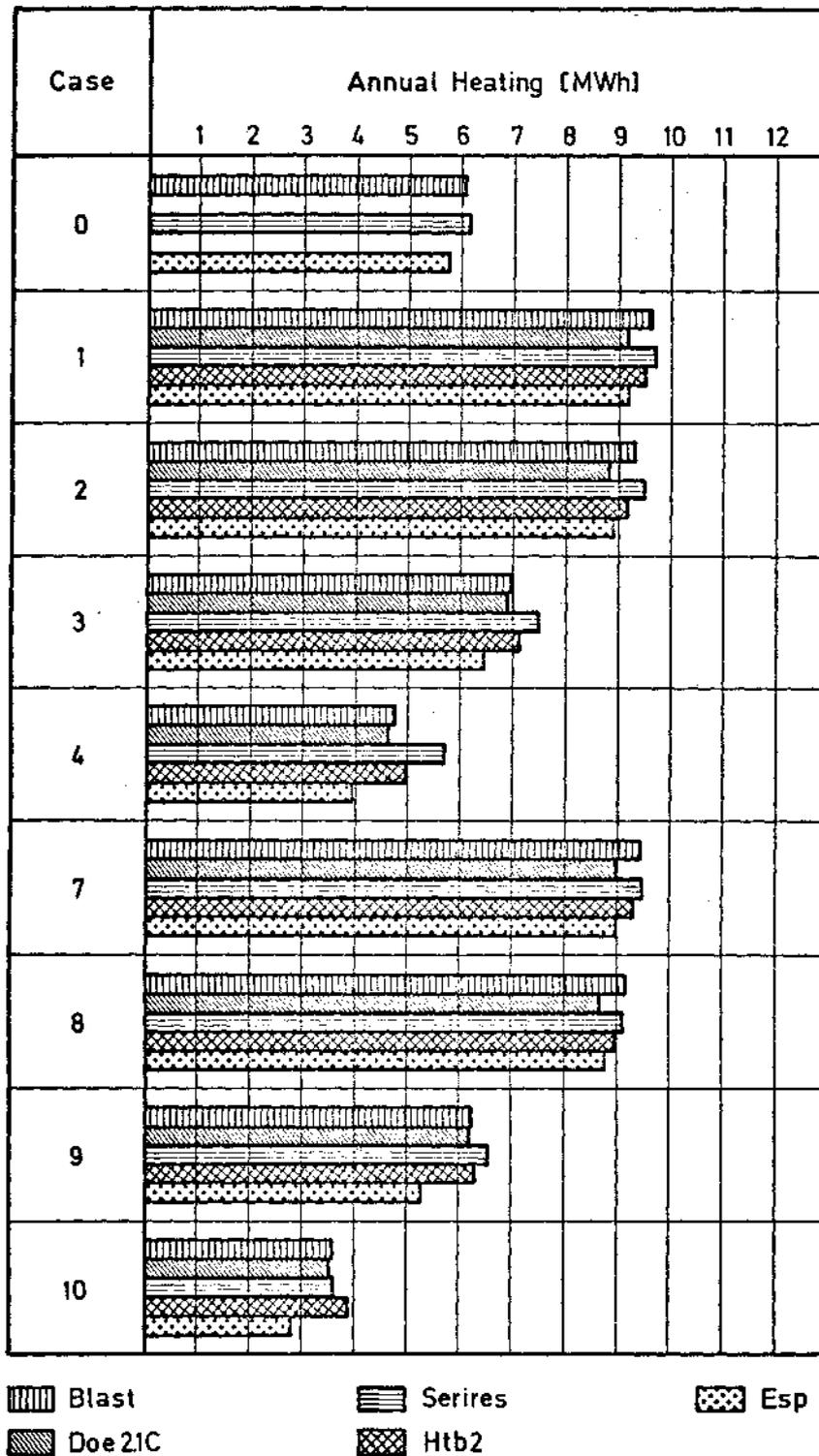
**Fig. 1** Annual heating loads of Phase I calculated by detailed building energy analysis simulation models with weather conditions of DENVER.
