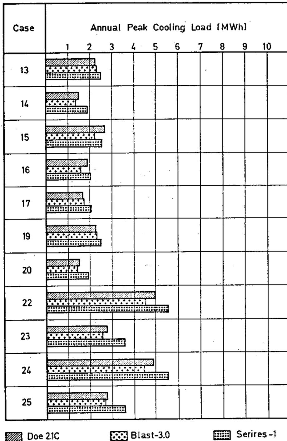
**Fig. 39** Annual peak cooling loads of Phase II calculated by detailed building energy analysis simulation models with weather conditions of DENVER.
