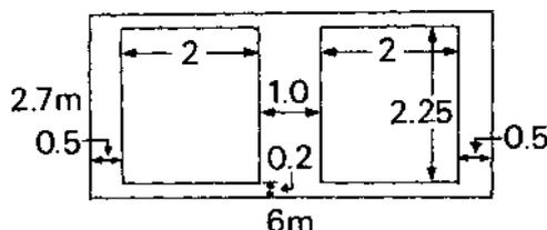
Figure A2: Glazing on South wall.
