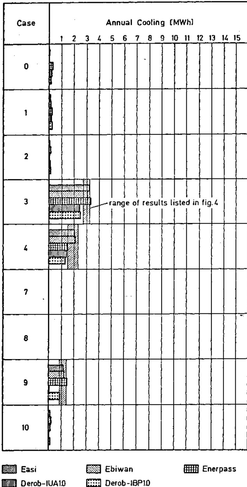
**fig. 20** Annual cooling loads of Phase I calculated by design tools with weather conditions of COPENHAGEN. Hatched areas indicate the ranges of results obtained by detailed building energy analysis simulation models (BLAST, DOE 2.1C, SERIRES, HTB 2, ESP) in Fig. 4.
