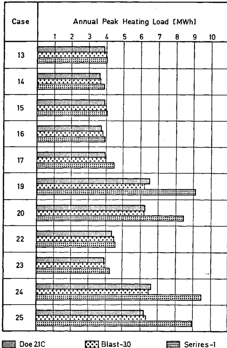
**Fig. 38** Annual peak heating loads of Phase II calculated by detailed building energy analysis simulation models with weather conditions of DENVER.
