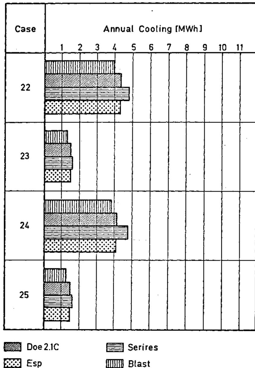
**Fig. 30** Annual cooling loads of Phase II calculated by detailed building energy analysis simulation models with weather conditions of DENVER.
