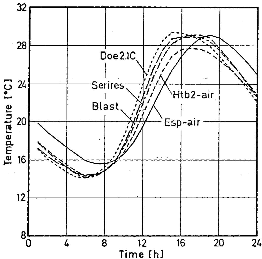
**Fig. 13** Hourly free-floating temperatures of Case 11 (lightweight building) calculated by detailed building energy analysis simulation models with weather conditions of DENVER, May 30.
