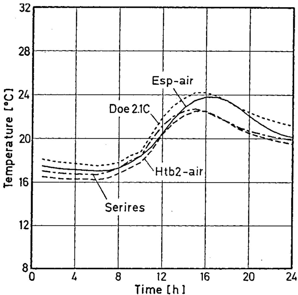
**Fig. 16** Hourly free-floating temperatures of Case 12 (heavyweight building) calculated by detailed building energy analysis simulation models with weather conditions of COPENHAGEN, May 30.
