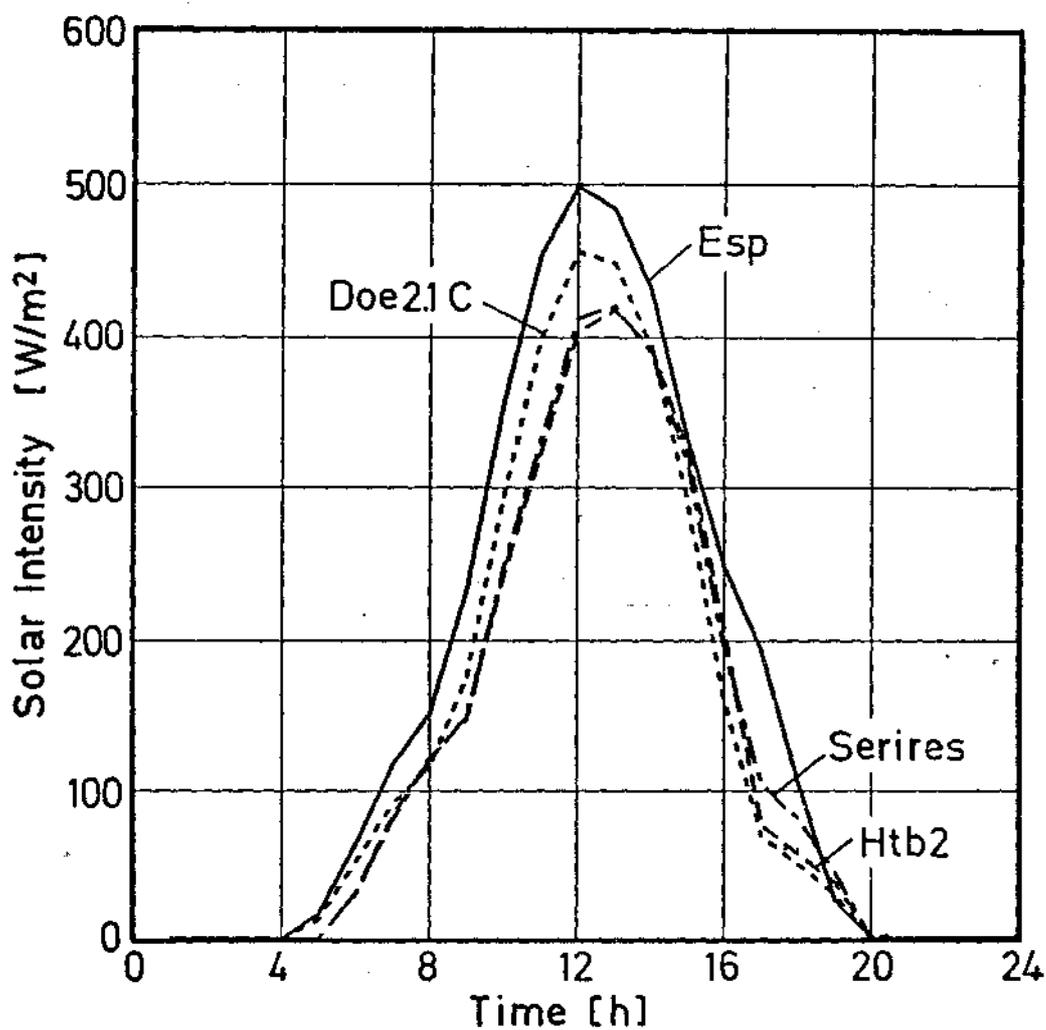
**fig. 9** Hourly solar radiation incident on the external south facing surface calculated by detailed building energy analysis simulation models with weather conditions of DENVER, May 30.
